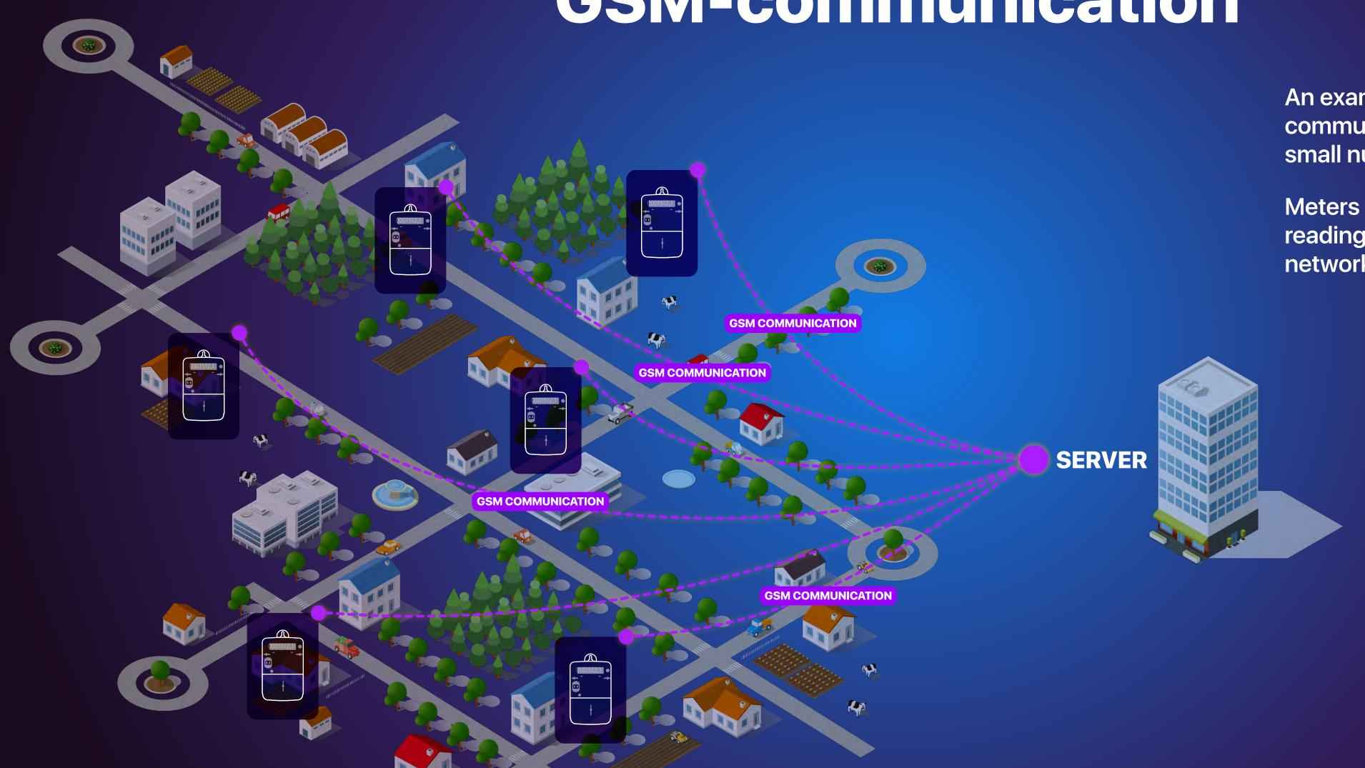
An example of a system using GSM communication for a remote village with a small number of consumers.
